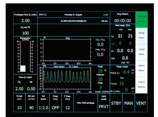
Siesta i TS display in PRVT mode with Neonatal settings
